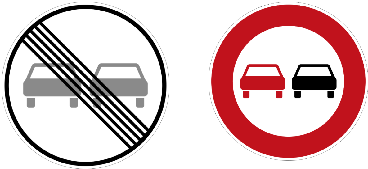
Image 7: Sign overtaking zone start (left), overtaking zone end (right) (Images not to scale)
